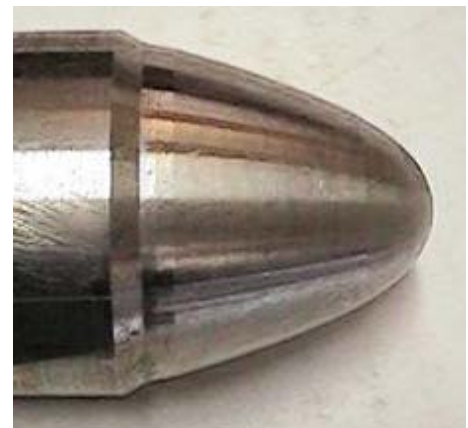
Linear Globe valve plug profile
