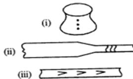
Formation of cracks in metal working process can be grouped as:i)Cracks at a free surface, as in a bulge in upsetting a cylinder or in edge cracking in rolling.
