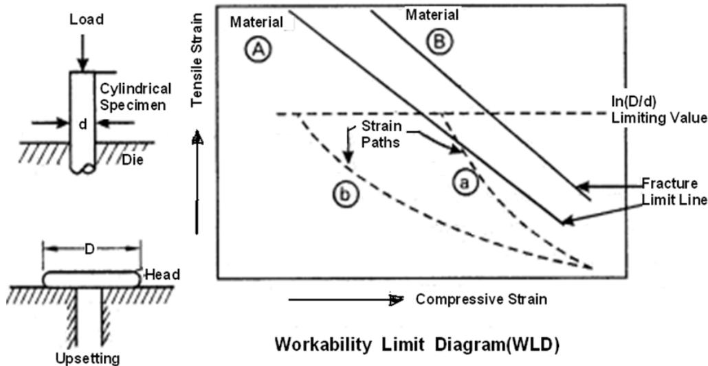
Now the process parameter represented by strain paths at potential fracture sites in the material is plotted. Strain paths can be determined either experimentally or by using FEA models. Soft materials like plasticine, lead or pure aluminium are taken and grids are placed on it and subjected to strain. The strain paths are determined from the path traced out by the deformation. These are then plotted in the diagram.
