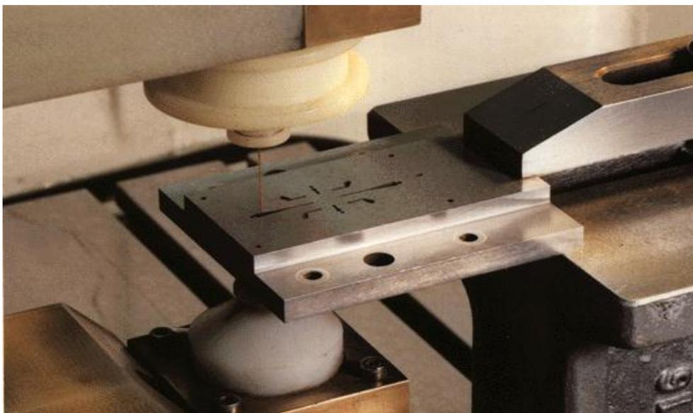
Figure 4: Wire erosion of an extrusion die
