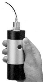
Figure 9.8 To calibrate a vibration measurement system, there are portable, battery-driven electrodynamic vibrators, that generate vibrations of a known frequency and amplitude. (Photo: Brüel & Kjær.)
