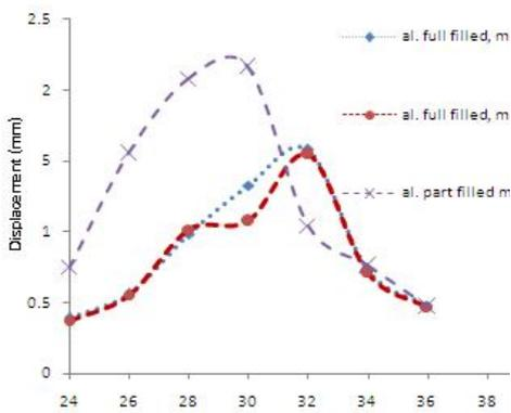
Fig. 5 Vibration spectra for partially filled beam
