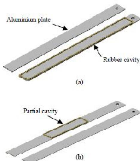
Fig. 1. Arrangement of aluminium beams
