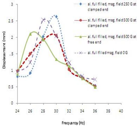
Fig. 4 : Vibration spectra for fully filled beam
