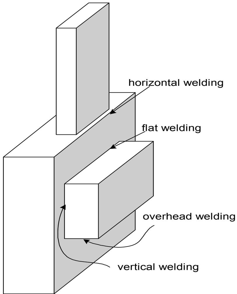
Fig. 23.4 Scheme of placement of components to be welded for different types of welding positions including overhead welding
