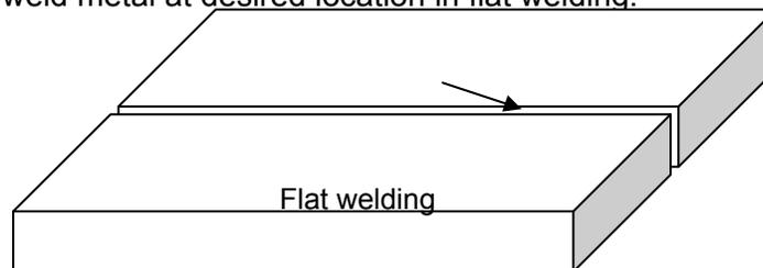
Fig. 23.1 Scheme of placement of components to be welded for flat welding
