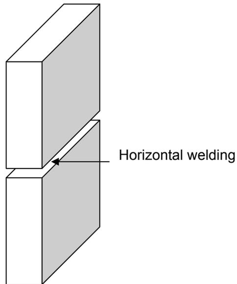
Fig. 23.2 Scheme of placement of components to be welded for horizontal welding
