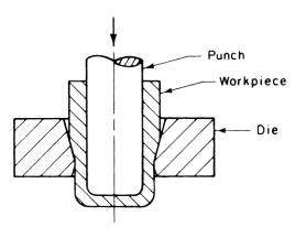
**Equipment.** Mechanical presses and hydraulic presses.
