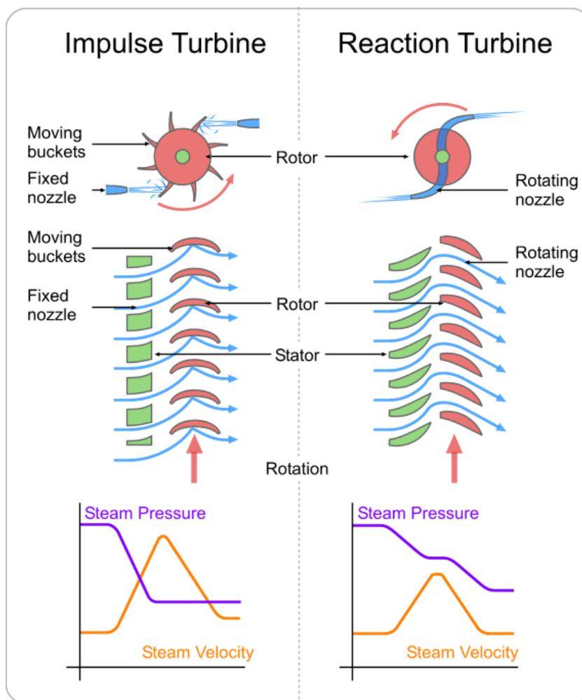
A device similar to a turbine but operating in reverse, i.e., driven, is a compressor or pump. The axial compressor in many gas turbine engines is a common example. Here again, both reaction and impulse
