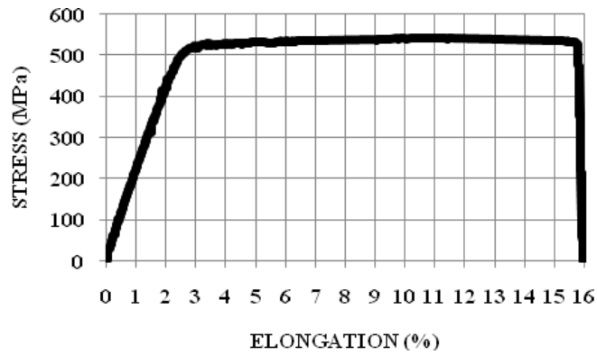
Fig. 3. Strain-stress diagram for AL 7017
