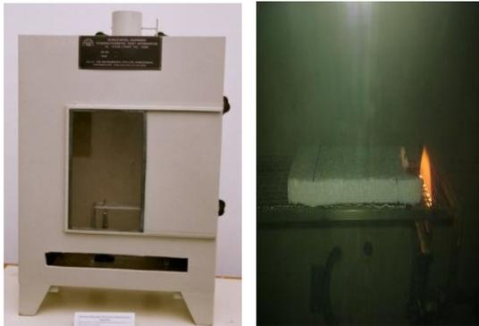
Fig.6 View of test chamber (left) and gauze holder (right)
