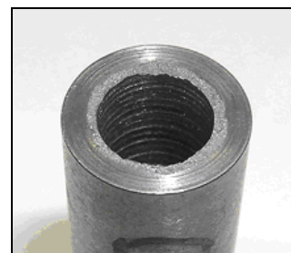
Fig. 6. Worked sample with X geometry drill tool
