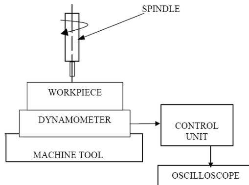
Fig. 6. Schematic representation of experimental set-up
