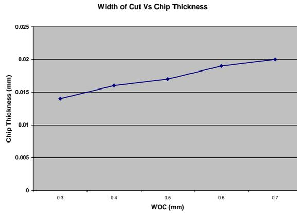
Fig. 10. Effect of width of cut on chip thickness
