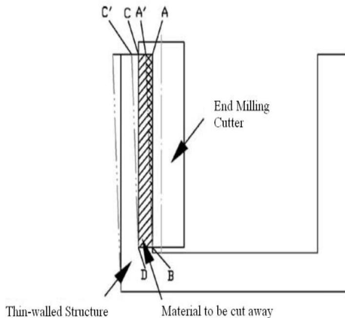
**Fig. 1. Machining sketch of the typical thin-walled structure.**
