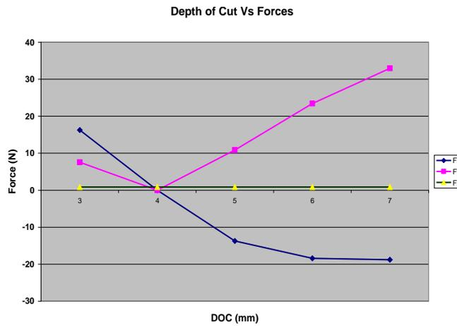
Fig. 11. Effect of axial depth of cut on cutting forces
