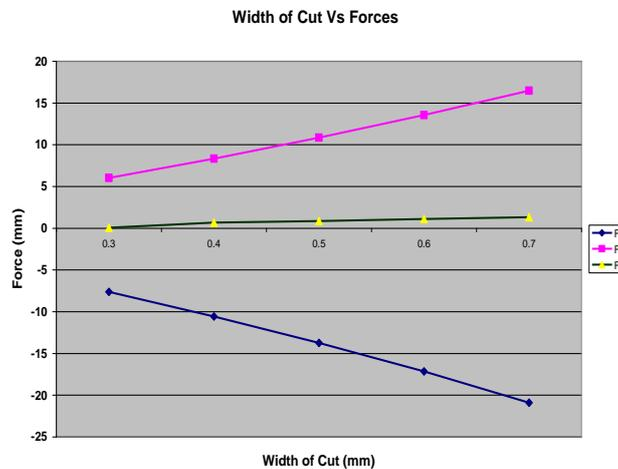
Fig. 9. Effect of width of cut on cutting forces
