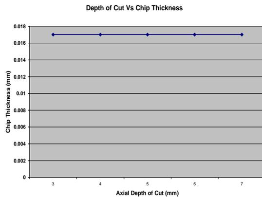
Fig. 12. Effect of axial depth of cut on chip thickness
