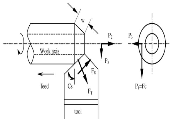
Fig. 3. Model for simple oblique cutting.
