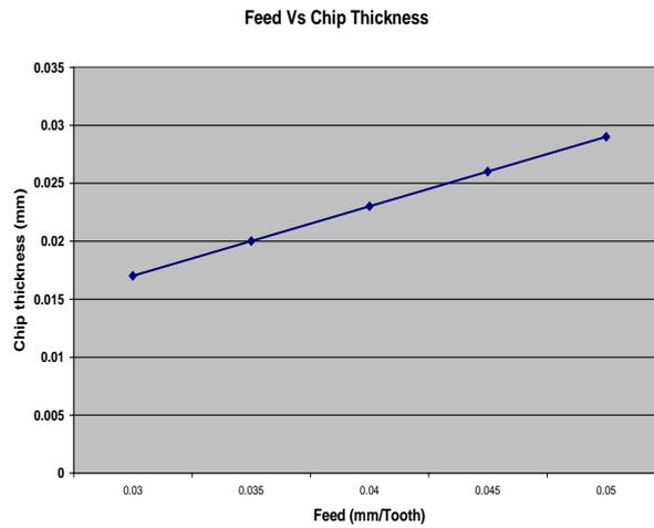
Fig. 8. Effect of feed on chip thickness
