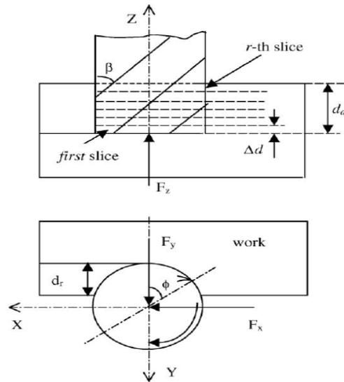
Fig. 2. Model for End milling Process
