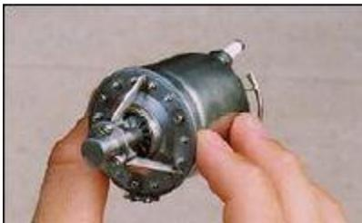
A micro turbine designed for DARPA by M-Dot
