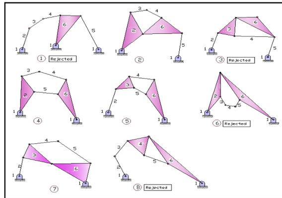
Fig. 17 : Corresponding linkage graphs for final enumeration results
