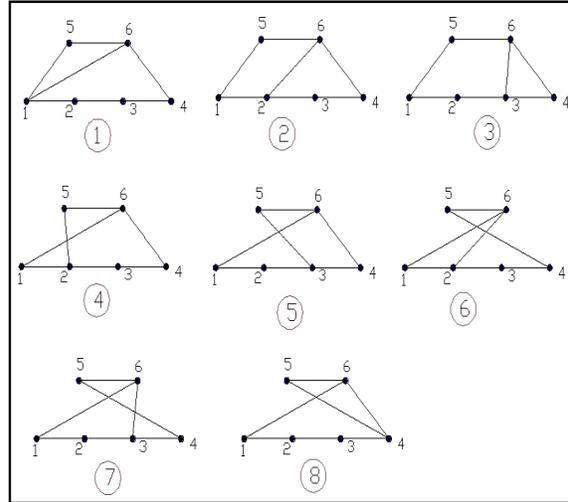
Fig. 16 : Final enumeration results for dependent link connection
