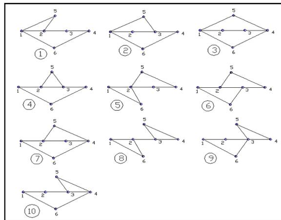
Fig. 8 : Final enumeration results for independent link connection
