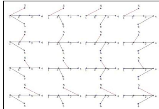
Fig.3 : Available candidates after adding the first two revolute joints for independent link connections
