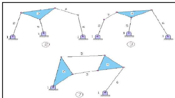
Fig. 11 : Available 6-bar mechanisms for independent link connection
