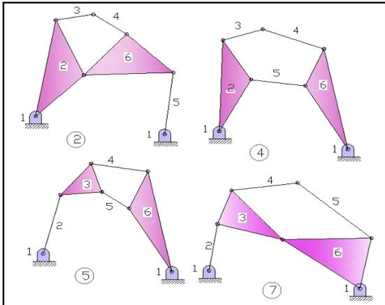
Fig. 18 : Available 6-bar mechanisms for dependent link connection
