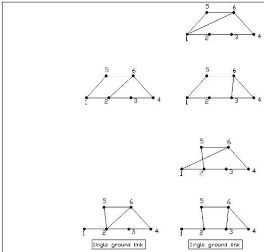
Fig. 15 : Detect graphs with single ground link
