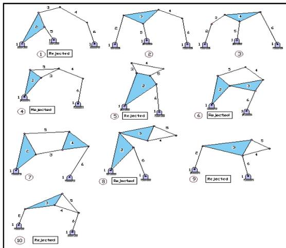
Fig. 10 : Corresponding linkage graphs for final enumeration results
