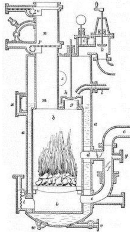
A diagram of Cameron's aero-steam engine, from an 1876 dictionary
