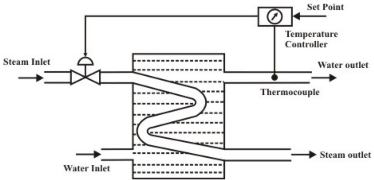
Fig. 1 Feedback temperature control of a heat exchanger
