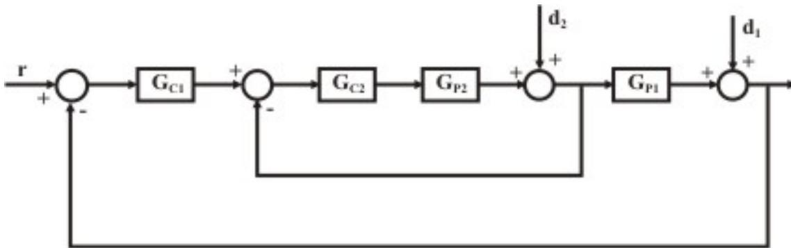
Fig. 5 Block diagram of Cascade Control System
