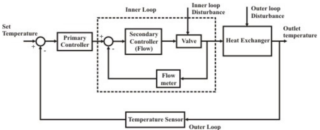
Fig. 3 Block diagram of a Cascade Control System
