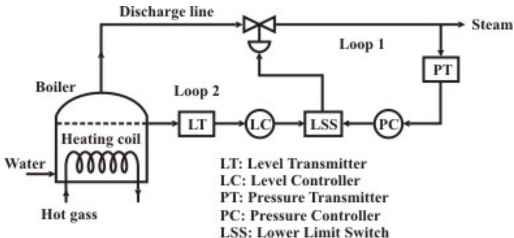
Fig. 6 Override control to protect a boiler system
