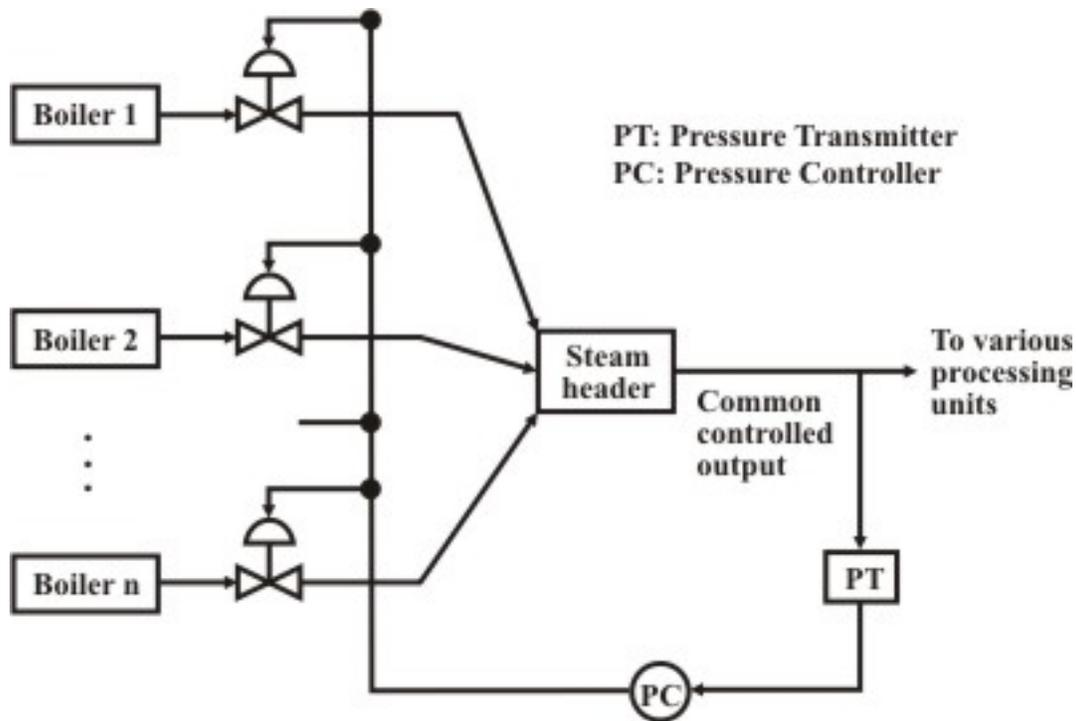
Fig. 7 Steam header with split-range control
