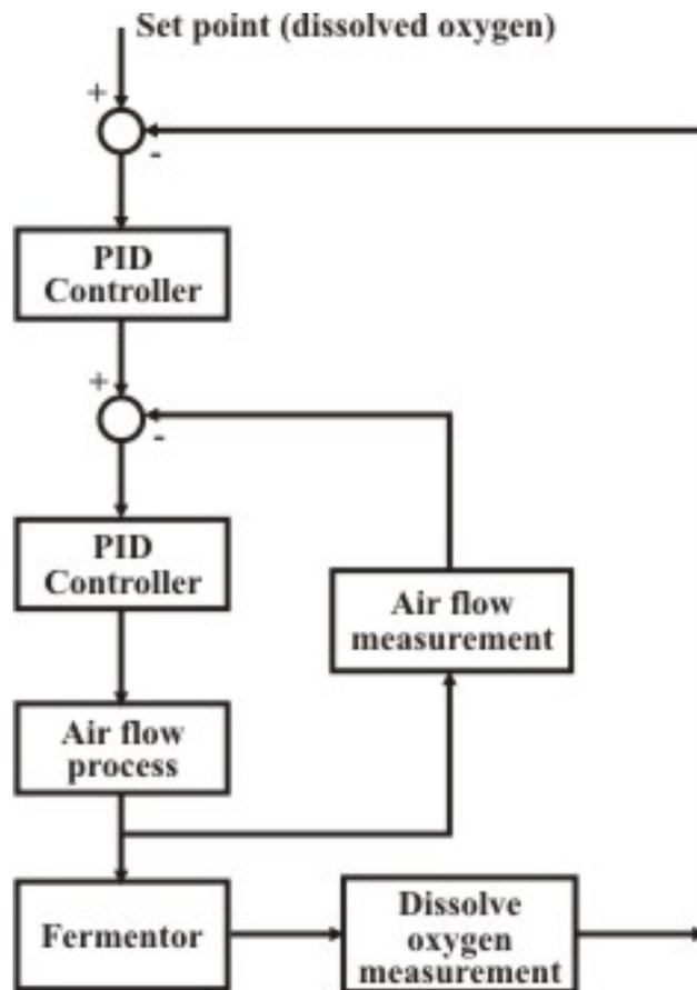
Fig. Q1 Control of a fermentation process
