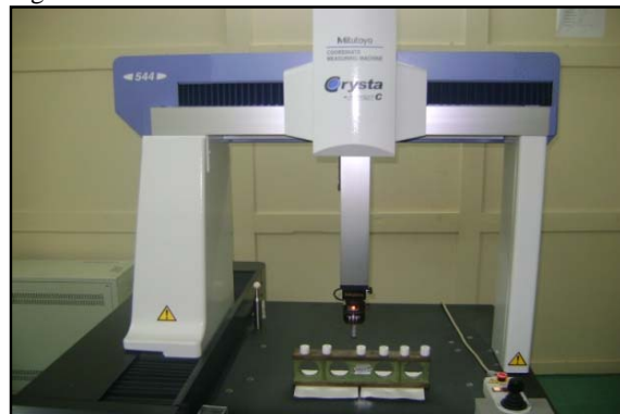
Fig. 2 : Measurement of Circularity error of the objects using CMM
