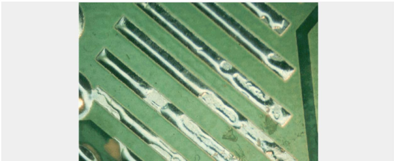
Note that a copper surface retains its colour, but one that has been wetted by solder will never become a clean copper surface again, because a diffusion layer has been formed.
