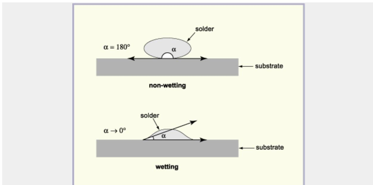
The solder should ideally wet the entire periphery of the termination to be soldered, and the thickness of the joint should increase evenly from the pad boundary to the termination: this presence of a 'fillet' helps confirm that the solder volume has been determined by joint geometry and surface tension and not constrained by undesirable factors.
