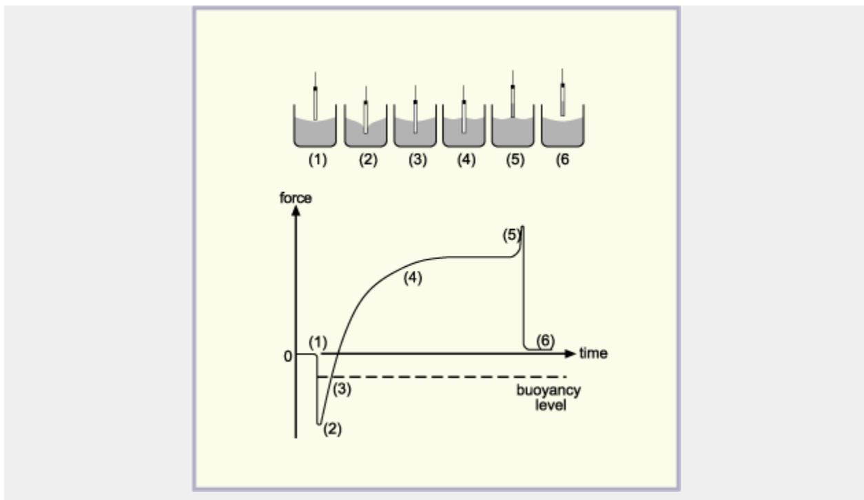
Some representative curves are also shown in Figure 3. In each case the full horizontal line represents the force at the start of the cycle and the dotted horizontal line the buoyancy level at which the wetting force is zero (a calculation based on the weight of solder displaced).
