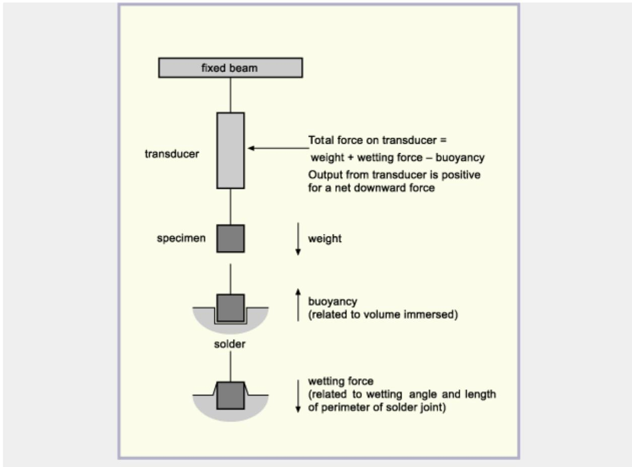
In Figure 2, the six stages of the testing of a readily wettable specimen are shown:
