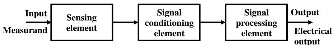
**Fig. 1 Elements of a measuring system.**
