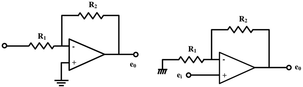
Fig. 7 (a) Inverting amplifier, (b) noninverting amplifier.
