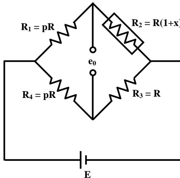
Fig. 2 Unbalanced D.C. bridge.
