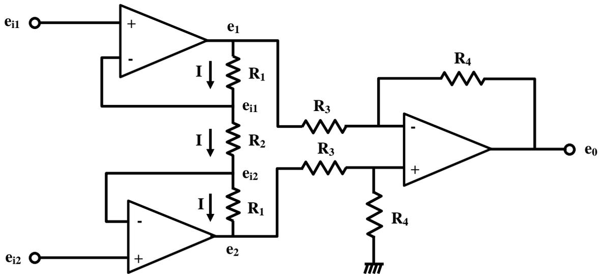
**Fig. 10 Three op. amp. Instrumentation Amplifier.**
