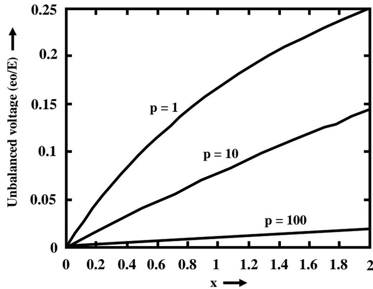
**Fig. 3 Bridge characteristics for different arms ratio.**
