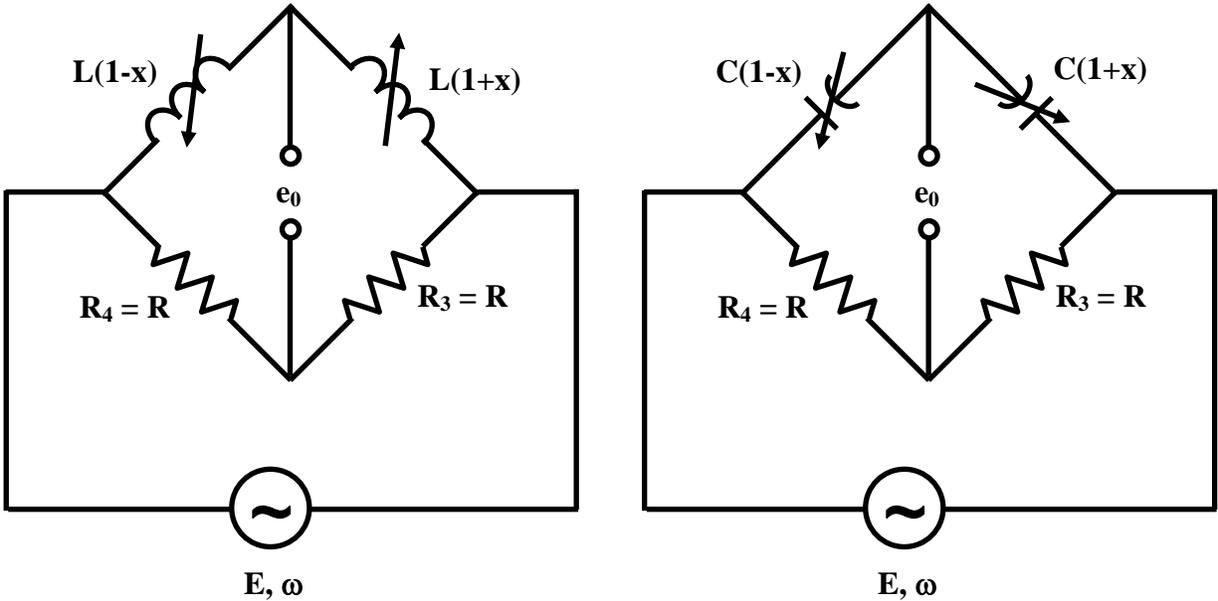
**Fig. 5 Unbalanced A.C. bridge with push-pull configuration: (a) for inductive sensor, and (b) for capacitive sensor.**
