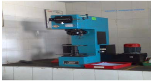
Fig.2 Experimental setup for Brinell Hardness strength test
