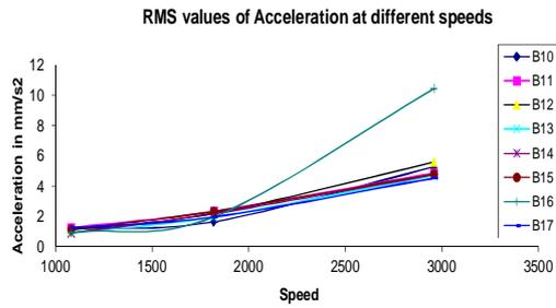
Graph- 3: RMS Acceleration Values VS. Speed in RPM
