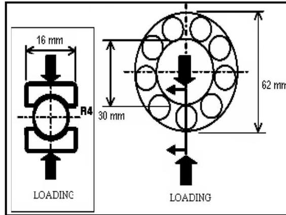
Figure 2- Bearing geometry
