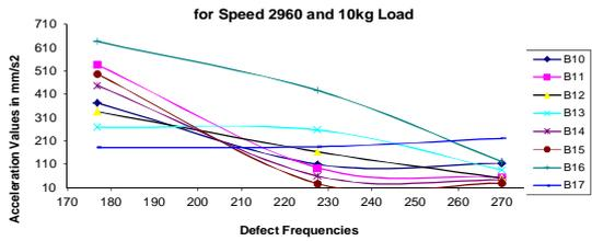
Graph- 3: Acceleration Values VS. Defect Frequency at speed 2960RPM
