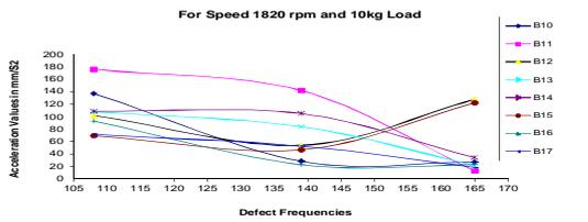
Graph-2 : Acceleration Values VS. Defect Frequency at speed 1820RPM
