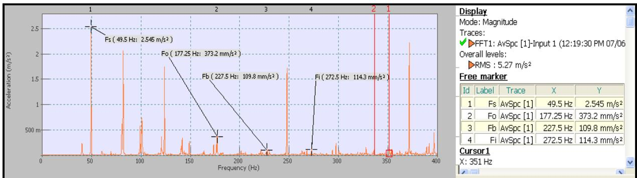
Figure 4. Signatures of Bearing Lubricated with Clean Grease
