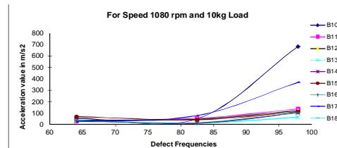
Graph- 1: Acceleration Values VS. Defect Frequency
