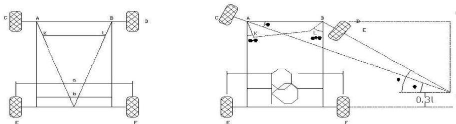
This mechanism is made of only turning pairs and is made of only turning pairs wear and tear of the parts is less and cheaper in manufacturing. The cross link KL connects
