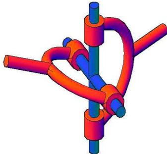
Hooke's joint used to connect two parallel intersecting shafts as shown in figure. This can also be used for shaft with angular misalignment where flexible coupling does not serve the purpose. Hence Hooke's joint is a means of connecting two rotating shafts whose axes lie in the same plane and their directions making a small angle with each other. It is commonly known as Universal joint. In Europe it is called as Cardan joint.
