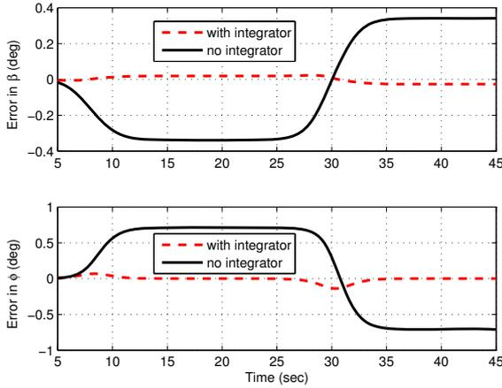
Fig. 3. Recovery of asymptotic regulation with conditional integrator.
