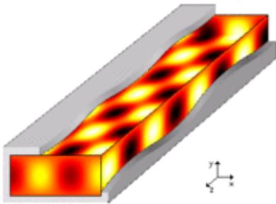
Electric field inside an x-band hollow metal waveguide.
