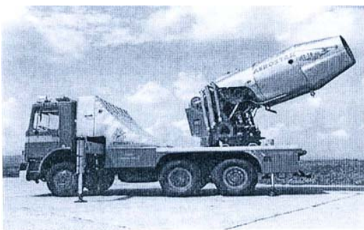
Fig. 2 A typical turbojet for land based activities
