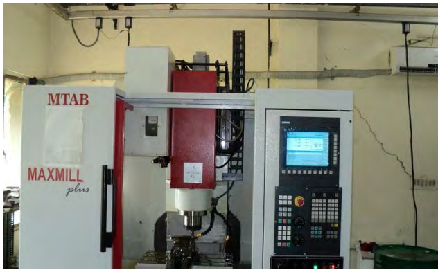
Fig.2: Experimental Set up of vertical CNC Drilling machine
