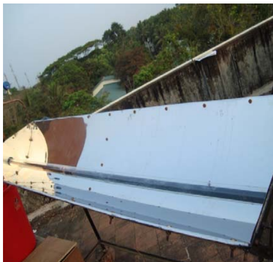
Fig. 3 Parabolic solar concentrator
