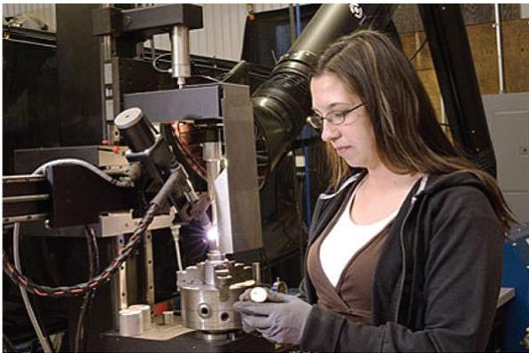
Figure 2. Fusion welded seams are TIG (Tungsten Inert Gas) welded.
