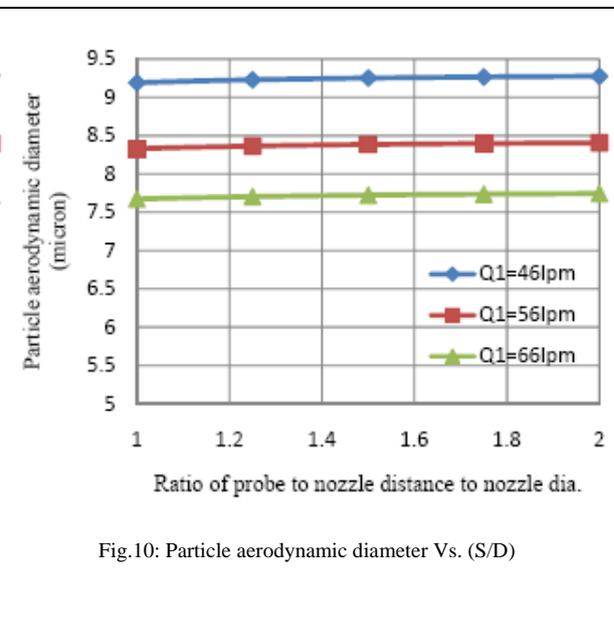
It is clear from Eq.3.12 that the effect of (D) on aerodynamic diameter of particles is the reverse of (Q<sub>1</sub>). The aerodynamic diameter of large particles was evaluated by Eq.3.22 at different levels of (Q<sub>1</sub>) and is featured in Fig.9 and Fig.10. Figure 9 and Fig.10 also show that the cut-off diameter increases as the total flow rate decreases which confirms the similarity of results available in literature.
