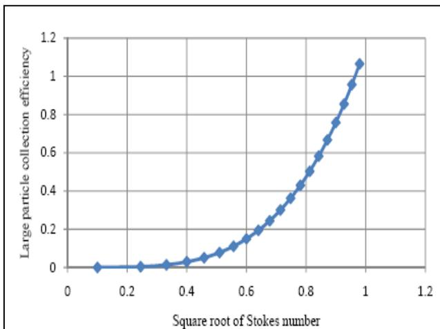
Fig.3: Large particle collection efficiency Vs.  $\sqrt{Stk}$
