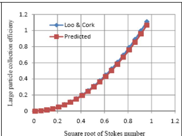
Fig.4: Large particle collection efficiency Vs.  $\sqrt{Stk}$
