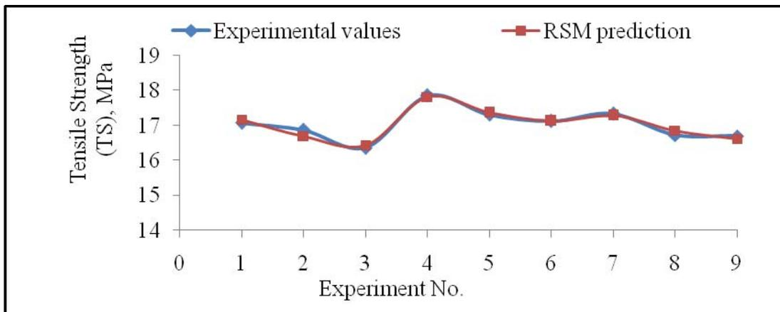
Fig: 15 Comparison of experimental values with RSM predicted values for Tensile strength (TS)
