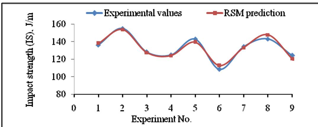
Fig: 17 Comparison of experimental values with RSM predicted values for Impact strength (IS)
