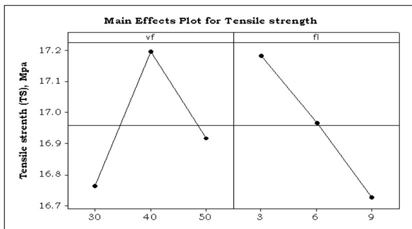
Figure: 6 Main effect plots for Tensile strength
