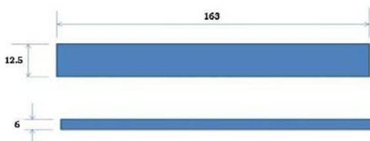
Fig:3 Specifications of Flexural test specimen
