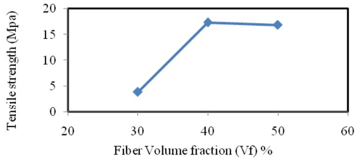
Fig: 9 Variation of Tensile strength with respect to fiber volume fraction
