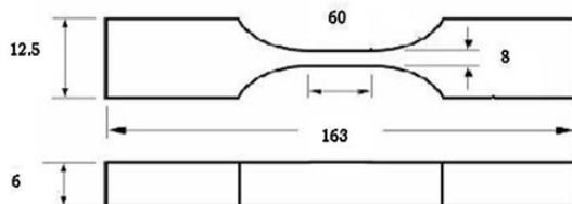
Fig:1 Specifications of Tension test specimen
