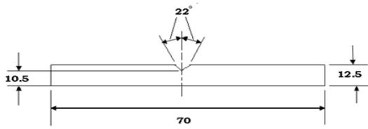
Fig:5 Specifications of Impact test specimen
