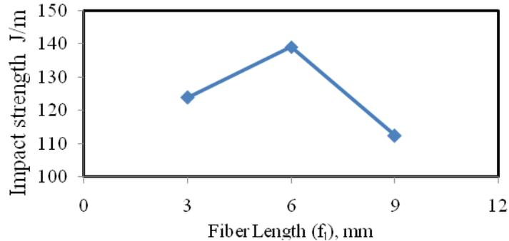
Fig: 14 Variation of impact strength with respect to fiber length.
