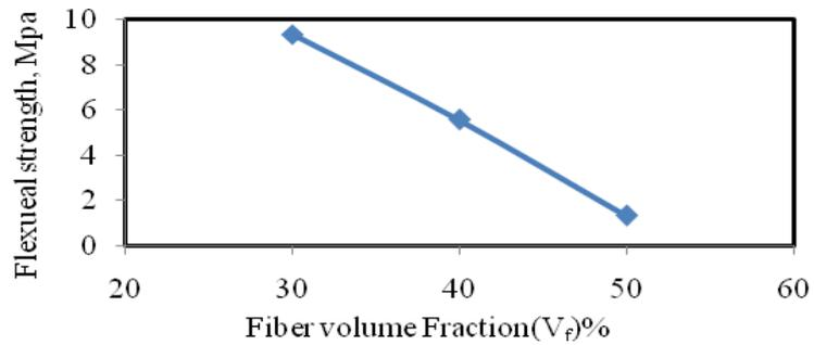
Fig: 11 Variation of flexural strength with respect to fiber volume fraction.
