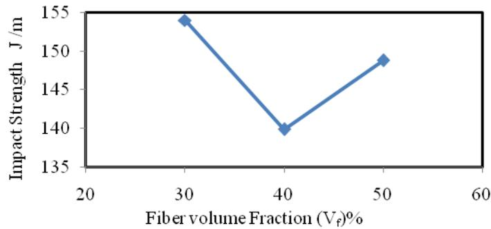
Fig: 13 Variation of impact strength with respect to fiber volume fraction.
