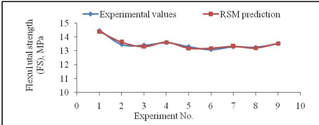
Fig: 16 Comparison of experimental values with RSM predicted values for Flexural strength (FS)
