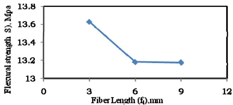
Fig:12 Variation of flexural strength with respect to fiber length.
