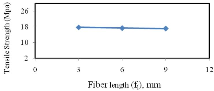
Fig: 10 Variation of Tensile strength with respect to fiber length.
