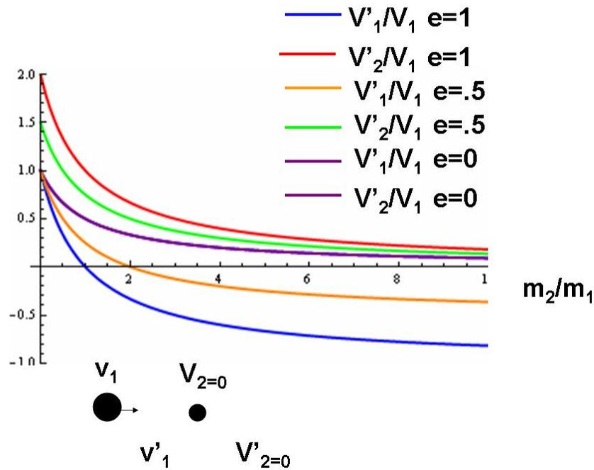
For  $e = 0$ , there is only one curve since the particles stick together:  $v'_1/v_1 = v'_2/v_1$ . For the elastic collision, note the result for equal masses:  $v'_1 = 0$  and  $v'_2/v_1 = 1$
