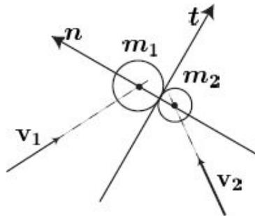
We write the equations of conservation of momentum in the tangent and normal directions. Since the force of contact is assumed to act along the normal direction, the conservation of linear momentum along the tangential direction implies
