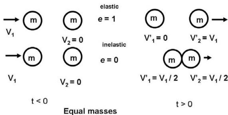
We consider two cases shown in the figure. In both cases one particle is at rest, the other approaching with velocity  $v_1$ . In one case, we assume an elastic collision,  $e = 1$ ; in the other a completely inelastic collision,
