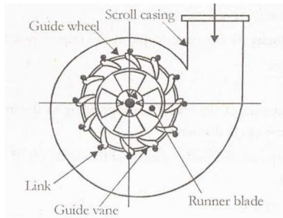
In the Kaplan turbine the runner has 4 to 6 blades attached to the hub or boss. The water enters the turbine in the axial direction. Since only a few blades are used the contact surface with water and hence the frictional resistance is reduced. The blades are made of stainless steel. The runner blades are so arranged that their angle of inclination can be adjusted while running. Hence the Kaplan turbine is also called variable pitch propeller turbine.
