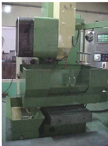
Fig. 1.3 A CNC Machine with an Automated Tool Changer and the Operator Console with Display for Programming and Control of the Machine
