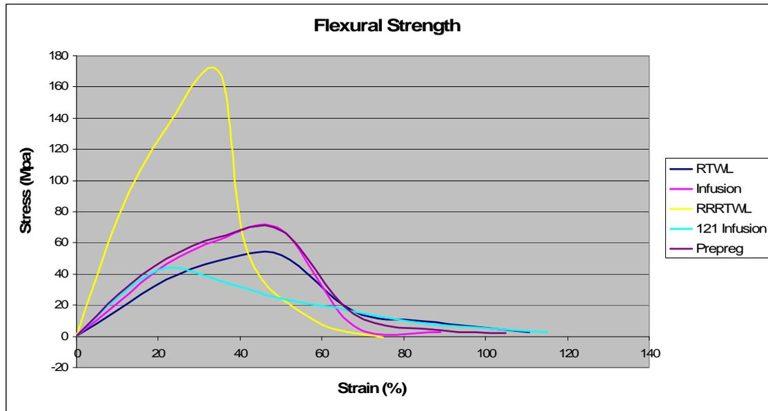
Figure 6: Flexural test results for infusion, pre-preg, RTWL, 121 infusion and RRRTWL
