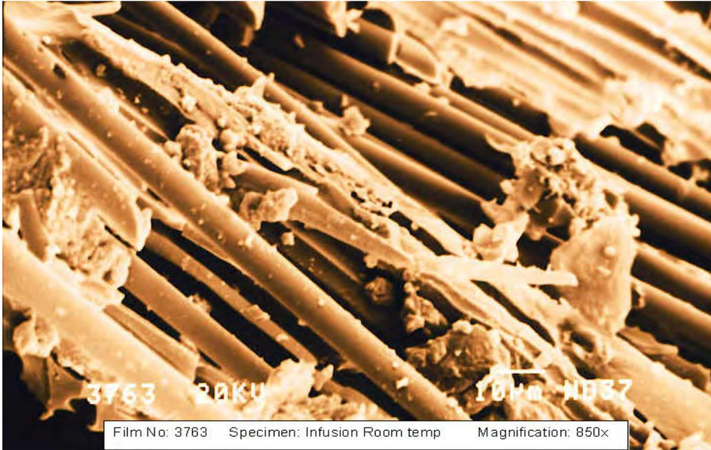
Fig. 2: SEM micrograph of 850-x magnification of the infusion repair method showing resin starved laminate.
