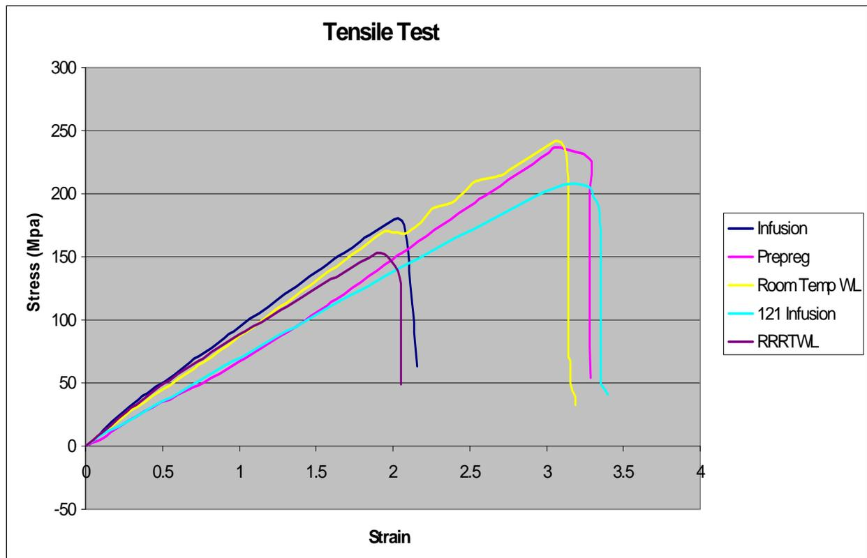
Fig. 1: Tensile test results for infusion, pre-preg, RTWL, 121 infusion and RRRTWL
