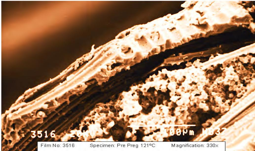
Fig. 4: SEM micrograph of 330-x magnification of pre-preg repair showing uniform breaking of the fibres. These are clean breakages of the glass fibres
