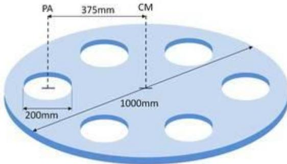
For an example of how to apply the parallel axis theorem, imagine that we are rotating a rotary table that is 1 meter in diameter, 10 mm thick, and made of steel. There are six holes cut into the table; each is 200 mm in diameter and the center of each hole is 375 mm from the center of the table.
