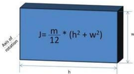
The mass of the side element is its volume times the density of aluminum ( $2660 \text{ kg/m}^3$ ) = 4.9 kg.
