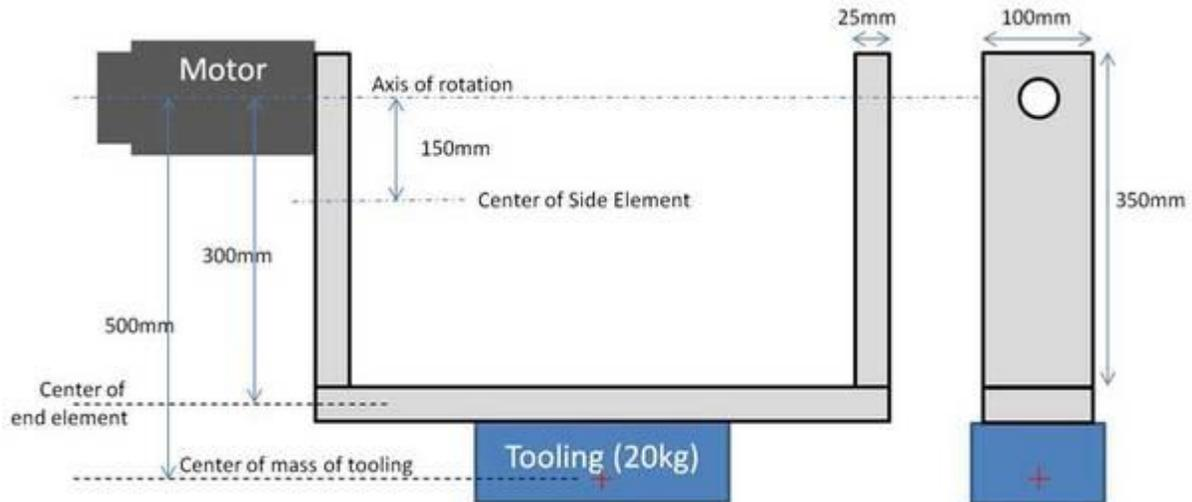
First, the inertia for each of the side elements rotated about its center is calculated:
