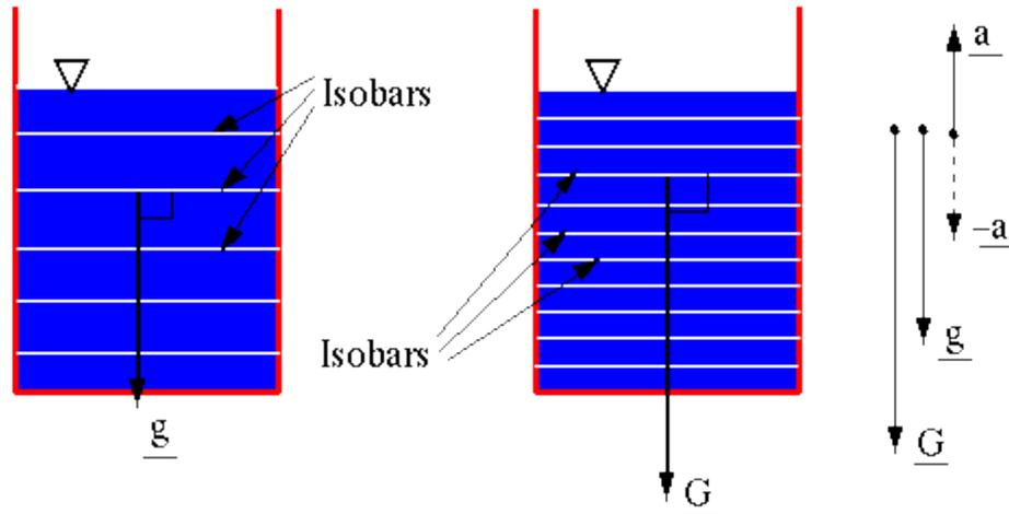
Here, the effective gravity is still downward, but of greater magnitude than  $g$ . The isobars are still horizontal surfaces as in hydrostatics. In fact, everything is identical to hydrostatics except for a larger gravity (pretend for example that the glass is sitting on the planet Jupiter). Our simple hydrostatic pressure relationship still applies, but with  $g$  replaced by  $G$ , and  $z$  replaced by  $s$ , i.e.
