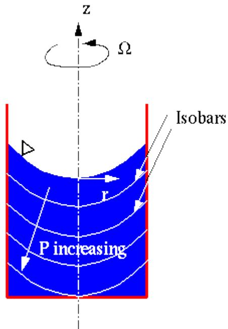
The free surface is of course an isobar, since its pressure is atmospheric. Pressure increases perpendicular to the isobars.
