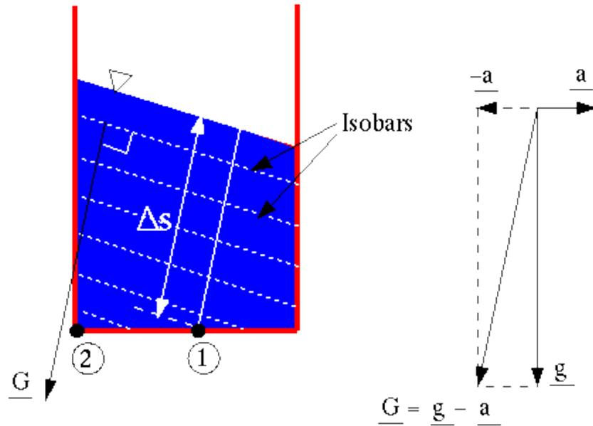
Now, since the effective gravity is tilted at some angle to the lower left, the isobars must be perpendicular to this direction. The isobars are thus tilted down and to the right as sketched. Note that the surface remains an isobar of constant pressure  $p_a$ , and is therefore also tilted as sketched. At some point 1 in the fluid, the pressure can be found from the revised hydrostatic pressure relationship as follows:
