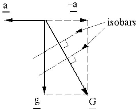
The local isobars around point B, being perpendicular to the local effective gravity vector, are thus tilted to the upper right even more severely than at point A. At the centerline (point C), the local acceleration is zero, and the effective gravity is identical to the standard gravity; isobars near the centerline of the rotating liquid are horizontal, just as in hydrostatics:
