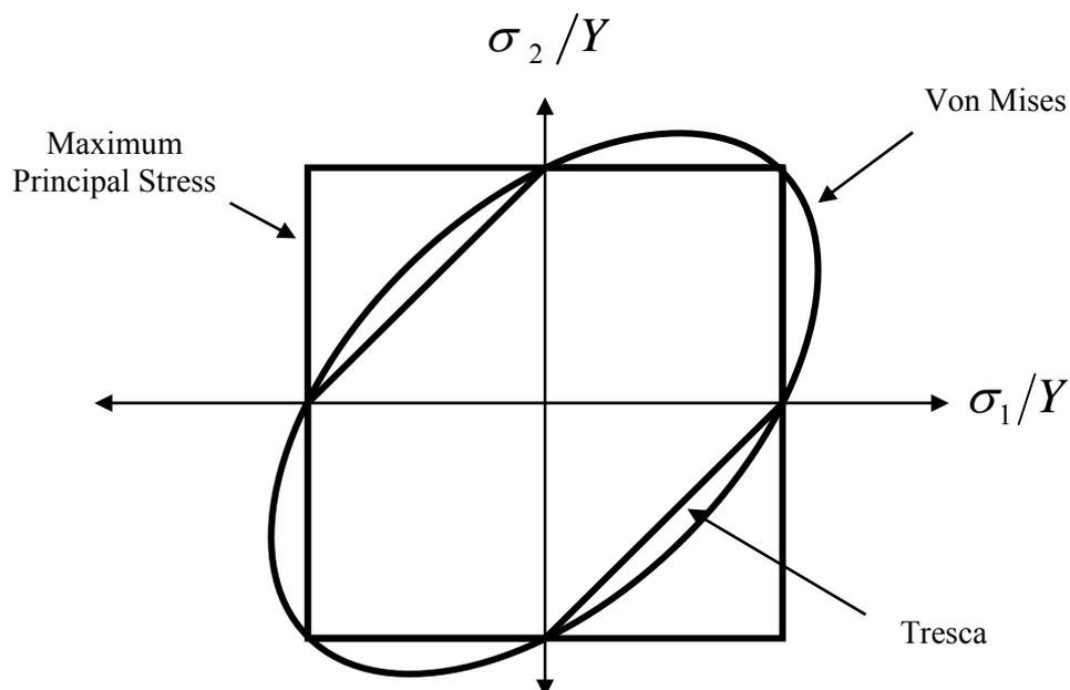
**Figure 9.1.4: Failure theories in stress space**
