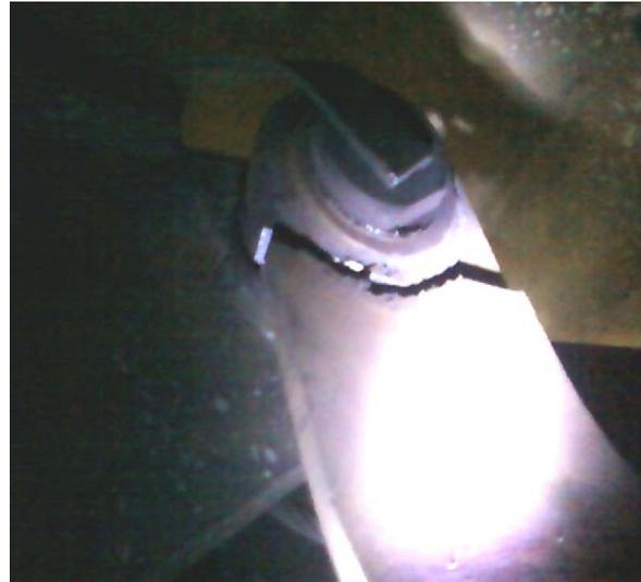
Figure 5: Present failure in Brake hanger
