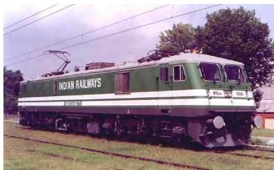
Figure 1: WAG-7 type Electric Locomotive
