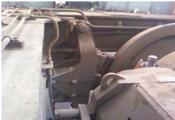
Figure 2: Brake hanger assembly
