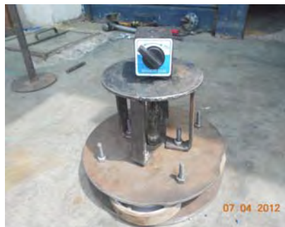
Figure 2.4 Front View of Lock Plate with magnet for attachment and deattachment of plate into machine
