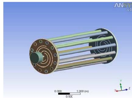
Ansys Assembly Of Linear Compressor
