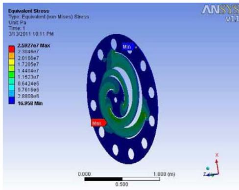
Fig.8 Equivalent Stress
