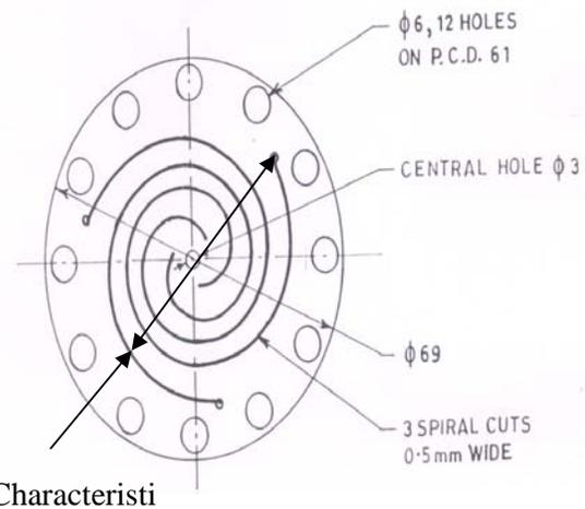
Fig 1 Typical flexure unit of the suspension system
