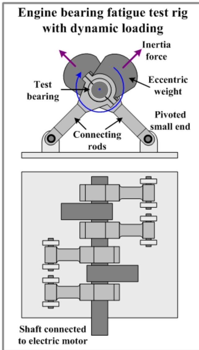
The principle of this type of Fatigue test rig is based on inertia forces generated by out-of-balance shaft.
