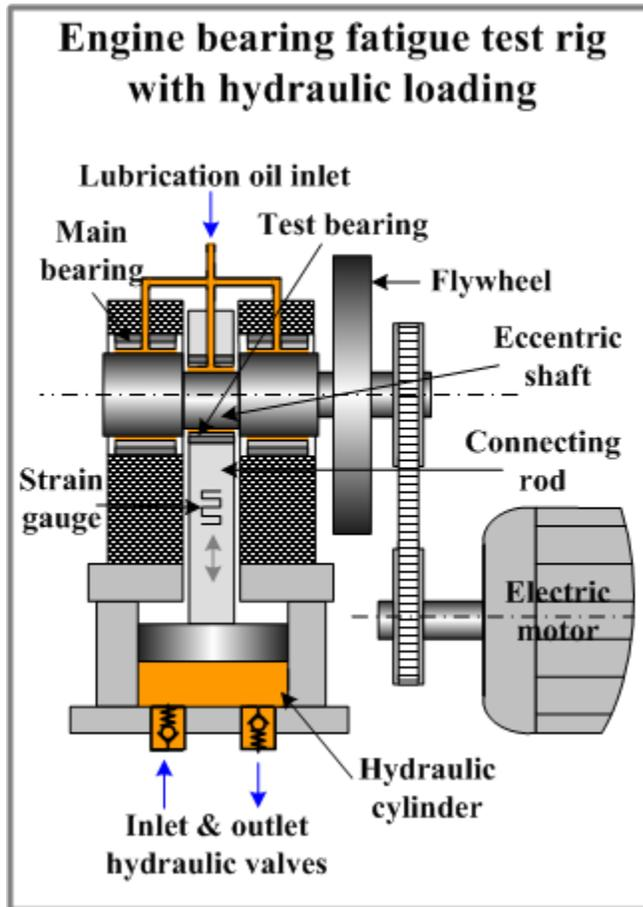
The principle of this type of Fatigue test machine is similar to internal combustion engines, in which pressure generated in the cylinders is transmitted to the bearings through the connecting rod.
