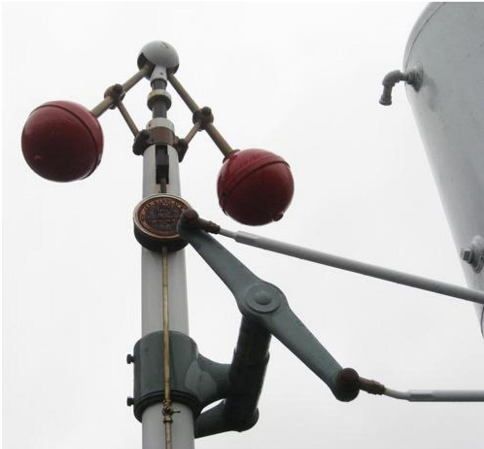
The governors are control mechanisms and they work on the principle of feedback control. Their basic function is to control the speed within limits when load on the prime mover changes. They have no control over the change in speed (flywheel determines change in speed i.e. speed control) within the cycle.
