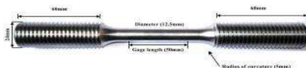
Fig. 2 Test specimen shape and dimension (KS B0801 10)
