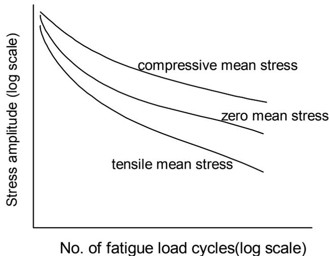
Fig. 27.6 Effect of type of stress on S-N curve
