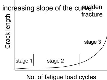
Fig. 27.1 Schematic of crack length vs. number of fatigue load cycles relationship
