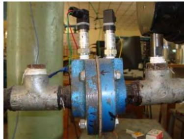
Figure 3. Orifice meter with pressure transducer
