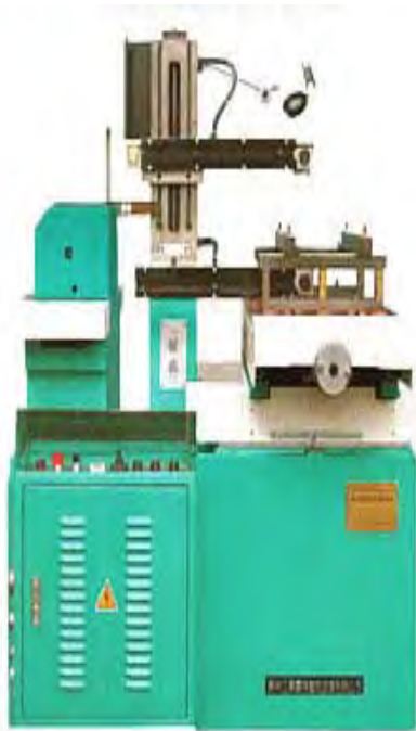
Figure -1: Concord 4-axis, CNC Wire Cut EDM
