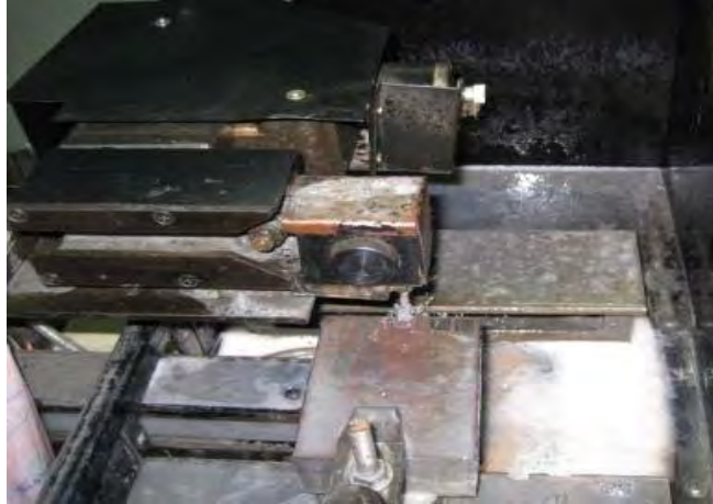
Figure - 3: Experimental Setup of the Wire-EDM
