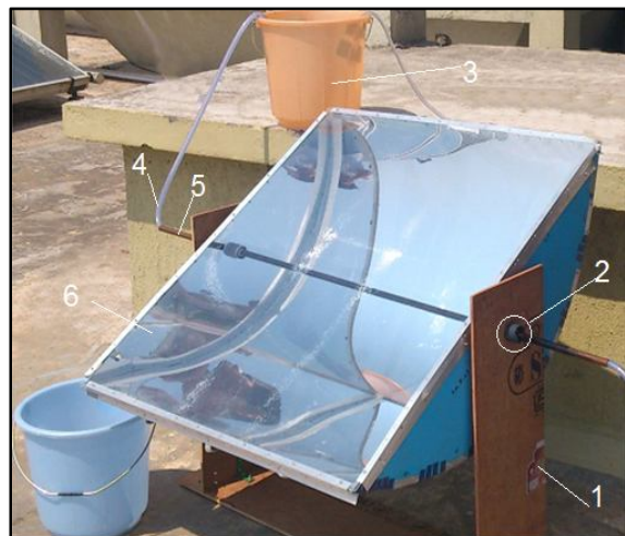
Figure 10: Thermal Collector with Thermosiphon Circulation
