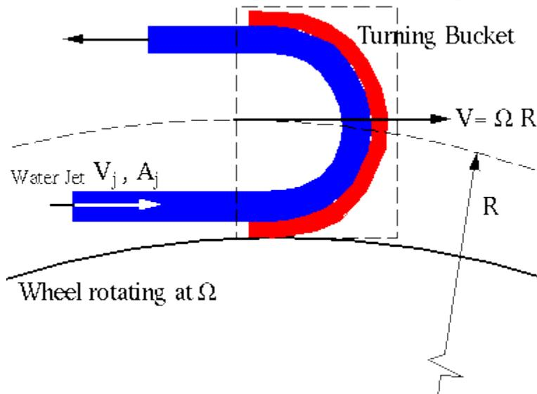
The turbine is spinning at a constant rotational speed.
