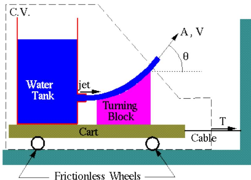
Known in this problem are the jet area  $A$ , the average velocity  $V_{av}$ , the jet deflection angle,  $\theta$ , and the momentum flux correction factor of the jet,  $\beta_{jet}$ . Also, frictionless wheels are assumed.
