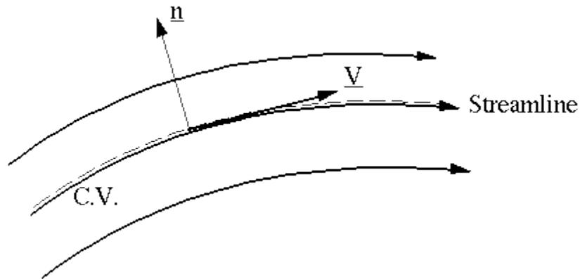
When you do this  $\underline{V} \cdot \underline{n}$  is equal to zero because they are perpendicular. This will cause the flux terms(mass, momentum, and energy) to be zero along the streamlines.
