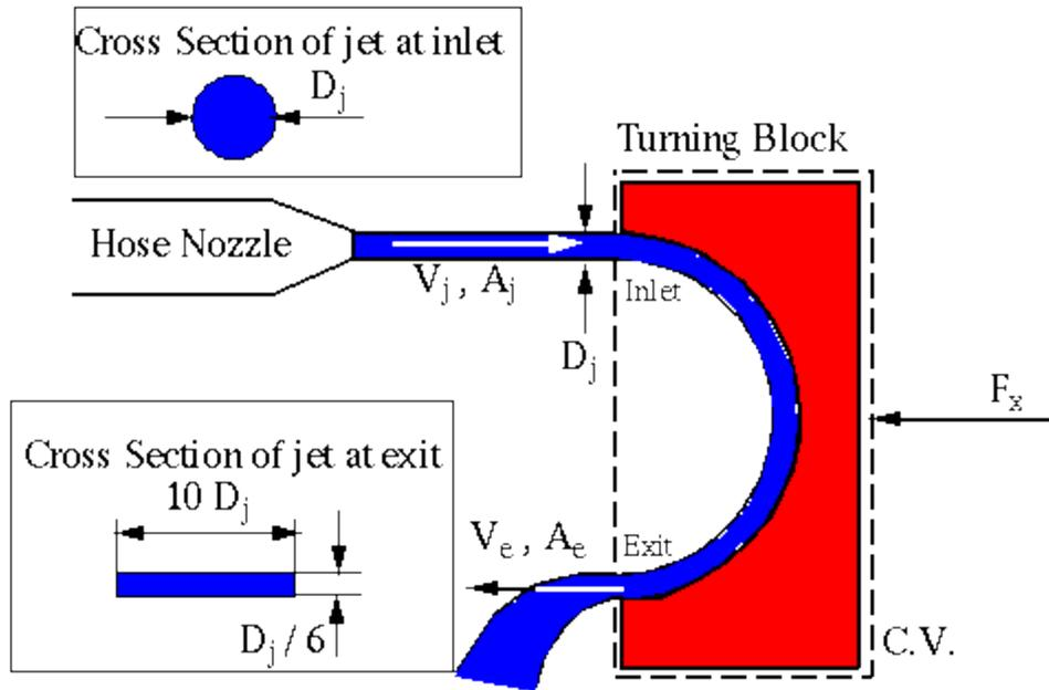
As the water leaves the block, the round jet flattens out and slows down due to friction along the wall. The water turns a full 180 degrees and flattens into a rectangle shape of thickness  $D_j/6$  and width  $10D_j$  in cross section. The flow is steady.
