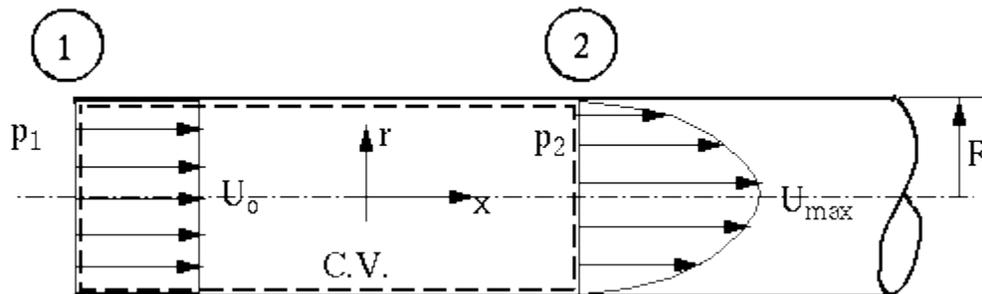
The inlet flow is uniform  $u_1 = U_0$ . The flow at section 2 is developed laminar pipe
