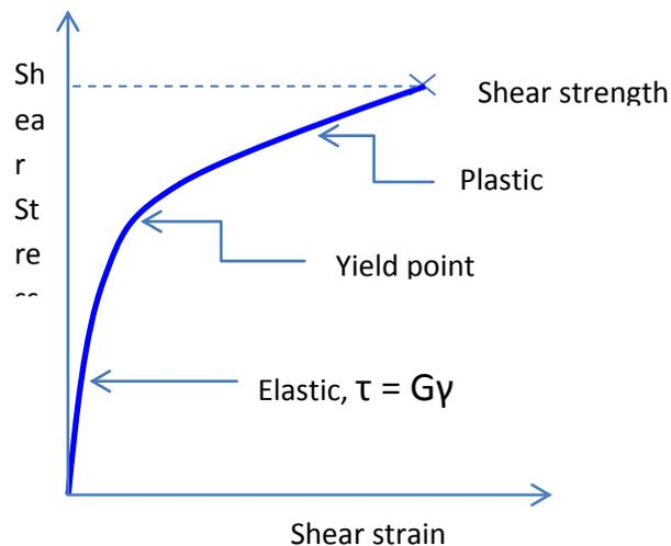
**Fig. 4.2.2: Shear stress- shear strain curve**
