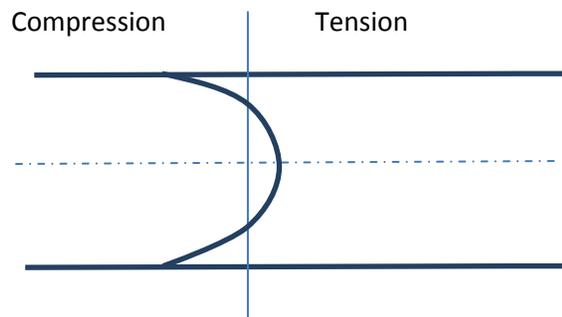
**Fig. 4.6.2: Residual stress in rolling**
