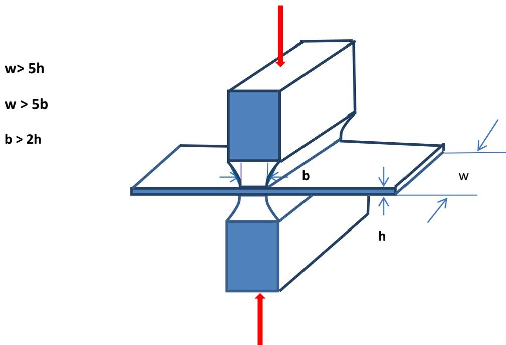
Fig. 4.1.2.1: Plane strain compression test for sheet metal
