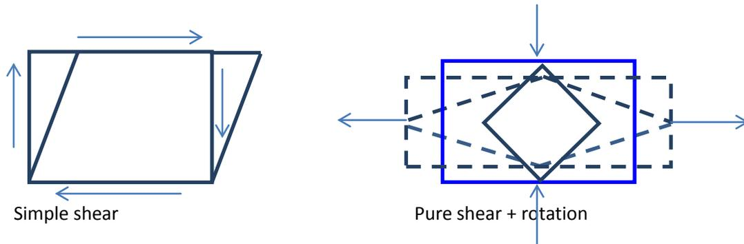
**Fig. 4.2.3: Shear Deformation**
