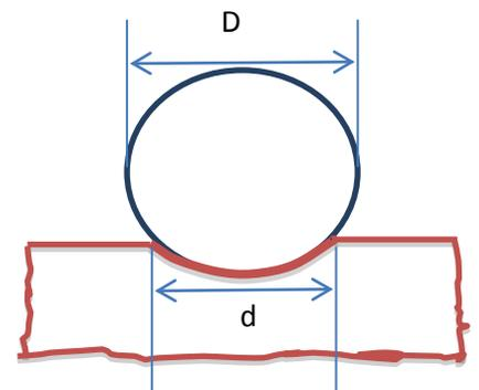
**Fig. 4.4.1: Indentation in Brinell test**
