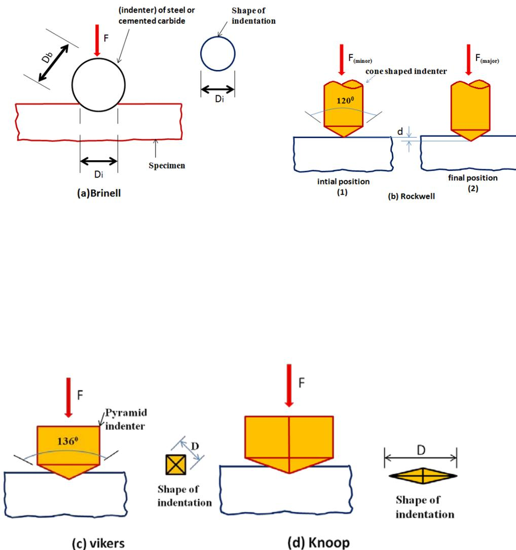
**Fig. 4.4.2: Indentation and indenters in various hardness tests**
